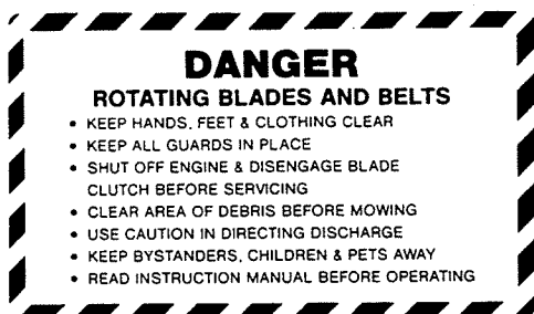
48073 Decal - Danger, Rotating Blades (Located On Cutter Deck Cover - Near Discharge Chute)
